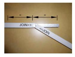
Step 3. Join the second channel to the CSJ by positioning the << JOIN of the channel at the centre of the CSJ, on an angle. Push the CSJ into the channel until you hear a 'click'.
