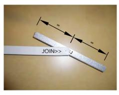
Step 2. Join the first channel to the CSJ by inserting the centre of the CSJ, on an angle, to the end of the channel where the JOIN>> text is marked.
