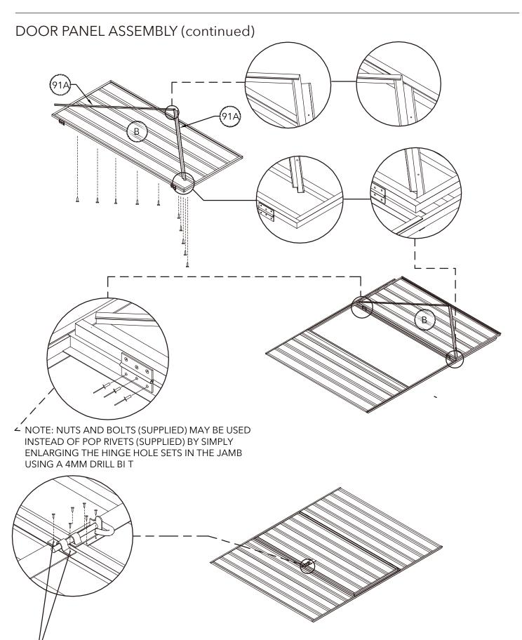
NOTE: The two holes required to connect the padbolt hasp for each door have not been pre-punched, to allow fo proper alignment. position each hasp centrally over the padbolt shaft, and drill 3mm holes and secure with screws
