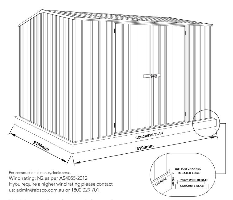
NOTE: This shed can be upgraded to wind rating: C1 as per AS4055-2012 with the additional purchase of a Cyclone Kit.
