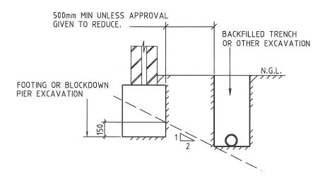
The contactor shall undertake investigatory localised excavations near existing footings to ascertain their depth prior to excavating adjacent to them. It is noted that excavating to a depth below that indicated above shall not be undertaken without the written approval from the engineer.
