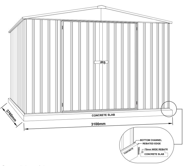
For construction in non-cyclonic areas Wind rating: N2 as per AS4055-2012. If you require a higher wind rating please contact us: admin@absco.com.au or 1800 029 701
