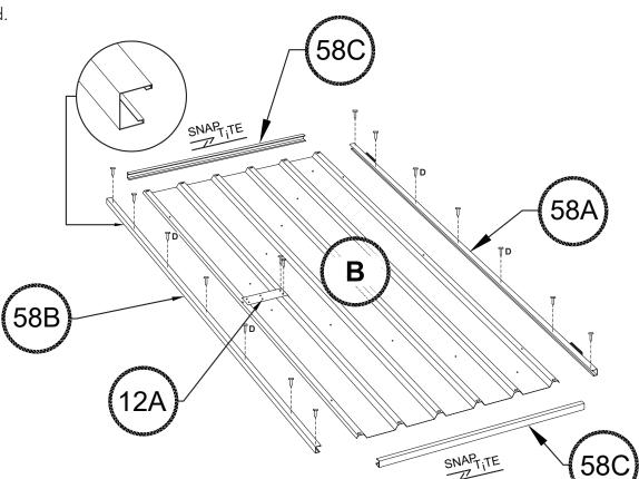
Vertical door channels are installed in the opposite orientation compared to the horizontal door channels.
